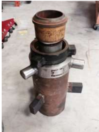
Figure 10: 4-1/2"XH (Box) Cross Over to Hammer Union
