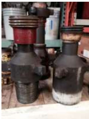
Figure 12: 3-1/2" (Pin & Box) Cross Overs to Hammer Unions
