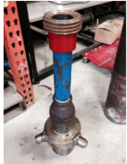
Figure 11: 4-1/2"XH (Pin) Cross Over to Hammer Union
