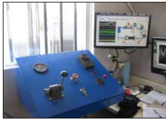
Figure 6: Flow Loop Controls and Data Monitoring
