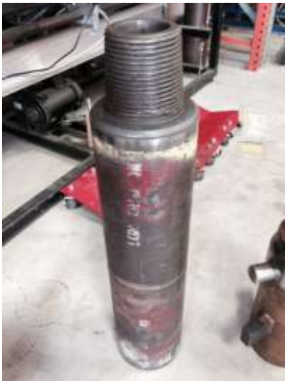
Figure 9: 4-1/2"XH (Pin) to 4-1/2"IF (Box) Cross Over
