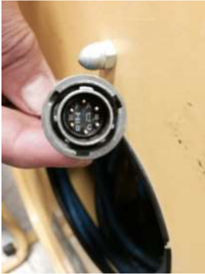
Figure 7: 6-Pin Male Connection to Surface Panel
