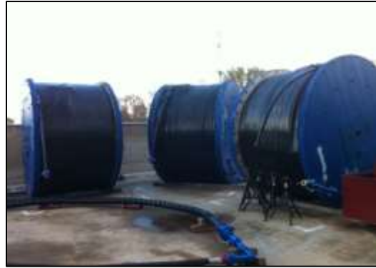
Figure 2: 2" Coiled Tubing Reels (14,000+ ft.)
