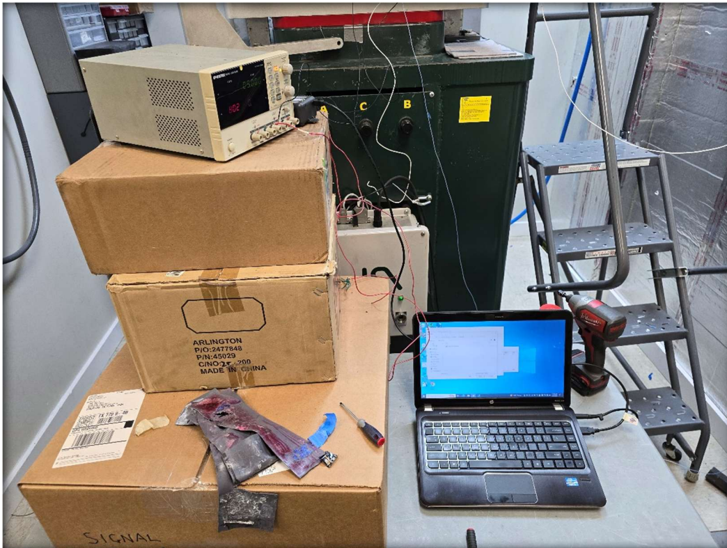
Figure 30: Test equipment used to monitor the UUT for shock testing
