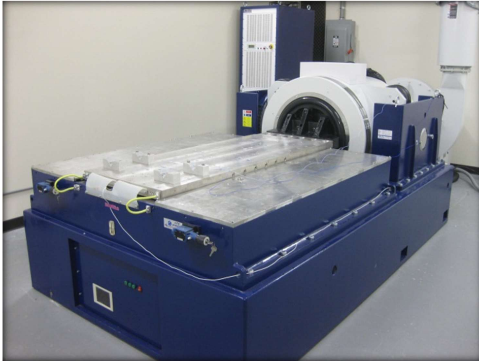
Figure 1: ETS-714, 15,400 lbf Shaker with 2'x5' slip table
