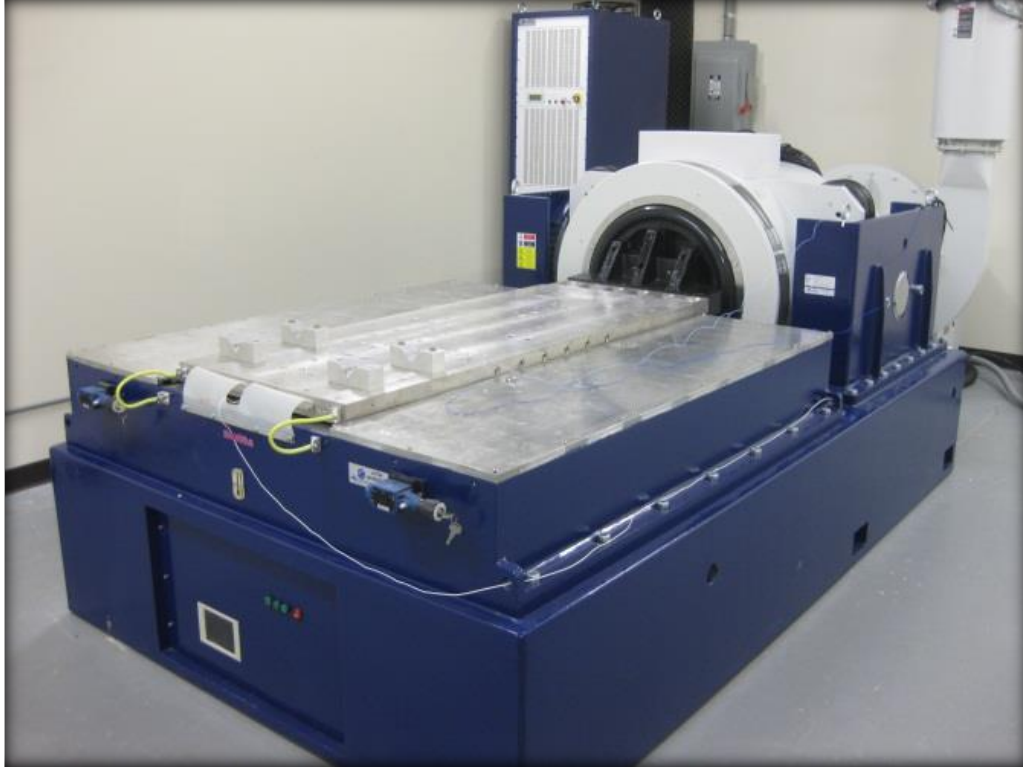
Figure x: ETS-714, 15,400 lbf Shaker with 2'x5' slip table
